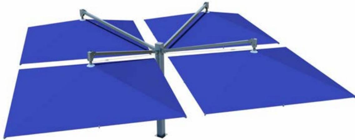
The Quadro mast combines 4 Amalfi parasols on a central mast thus rendering shadow to especially large areas up to 49 m<sup>2</sup>. The four canopies are fixed to the mast employing a bayonet suspension and can be opened separately from each other with 4 auto locking winches.
